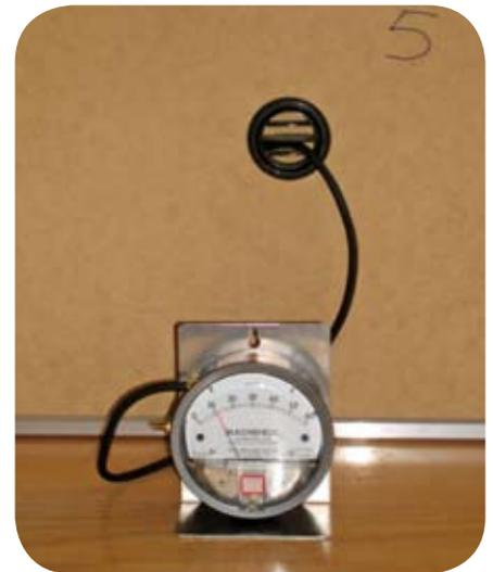
Figure 11 Pressure at 7.5L/s/diffuser
