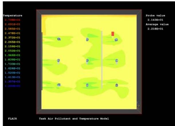
Figure 6: Temperature distribution for UCI Task Air conditioning.
