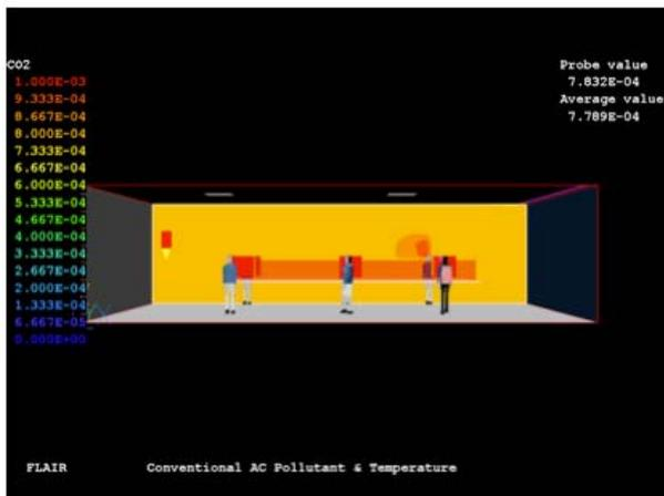
Figure 3: Carbon Dioxide levels approximating 780ppm in VAV office.
