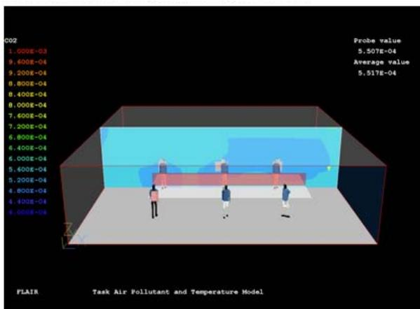
Figure 4: Carbon Dioxide levels approximating 550ppm in breathing zone with UCI Task Air.
