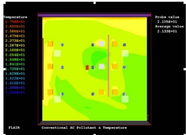
Figure 5: Temperature distribution in VAV office.
